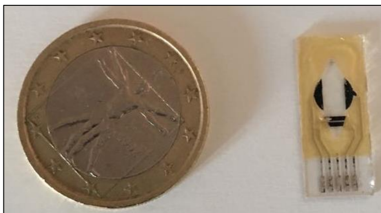
Figure 4-6 Chip after manufacturing. The TMMF defining the microfluidic channel is yellow, the sensing parts of the electrodes are black (coated) and the contacts are grey (uncoated). A one Euro coin is used as reference for dimensions.
