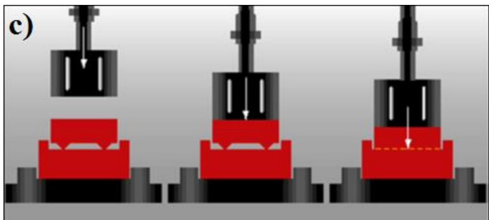
Figure 4-13 Alternative bonding technique. a) OSTe+ dual cure polymer chemical reaction scheme [117]. b) APTES/GPTES chemical reaction scheme [119]. c) Ultrasonic bonding process from Trackenmuller et al. [122].
