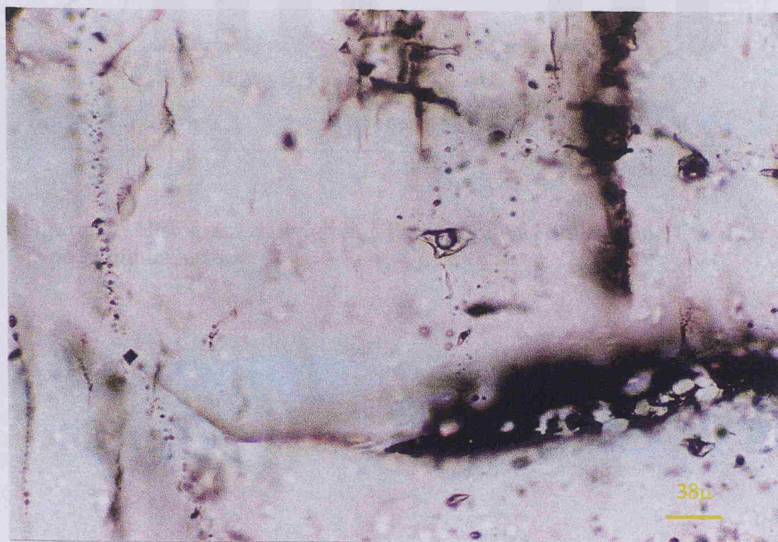
Plate 7.3: Variable \text{CO}_2/\text{H}_2\text{O} ratio in Type I inclusions indicating immiscibility. Note that some inclusions in (a) have been decrystallized to vapour phase before homogenisation.
