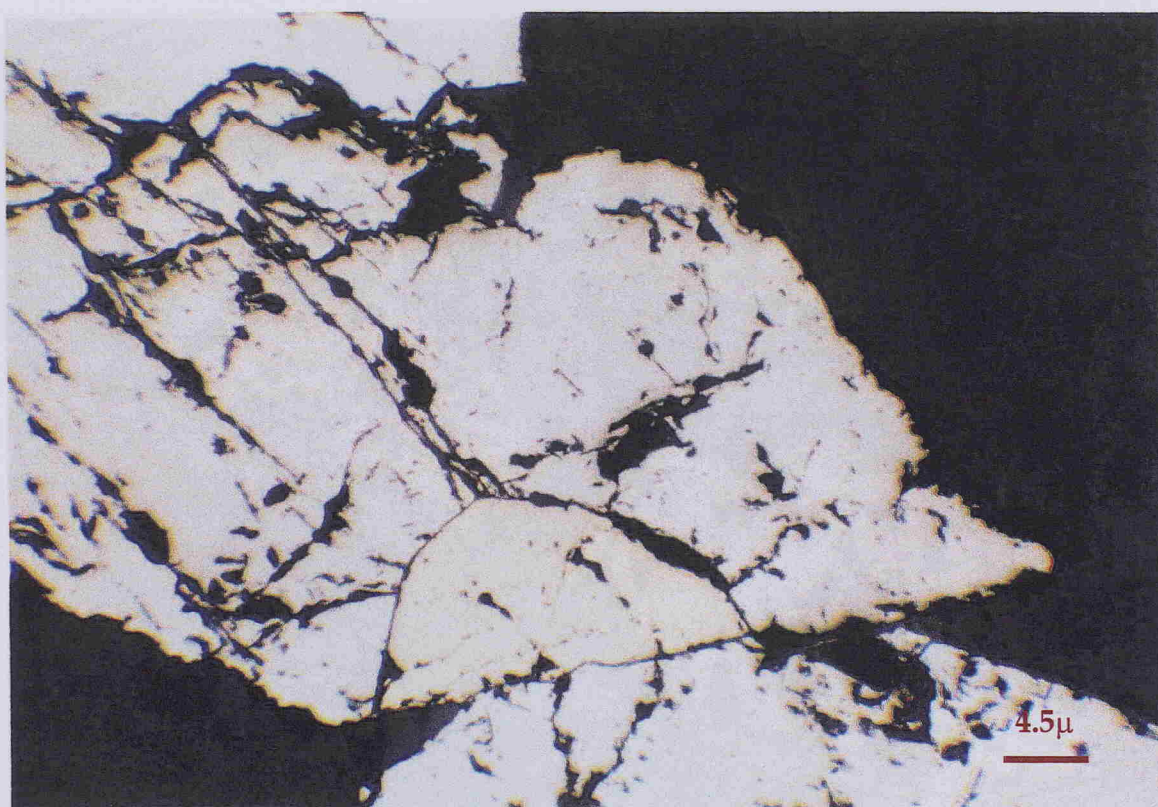
Plate 5.3: (a) Equilibrium deposition of arsenopyrite and pyrite (more yellow). (b) Intergrowth of arsenopyrite prisms and pyrite (more yellow).
