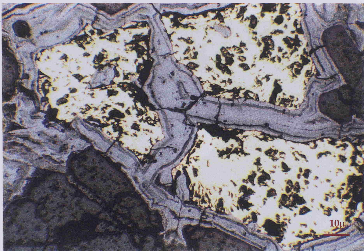
Plate 5.4: Oxidised chalcopyrite in goethite.
