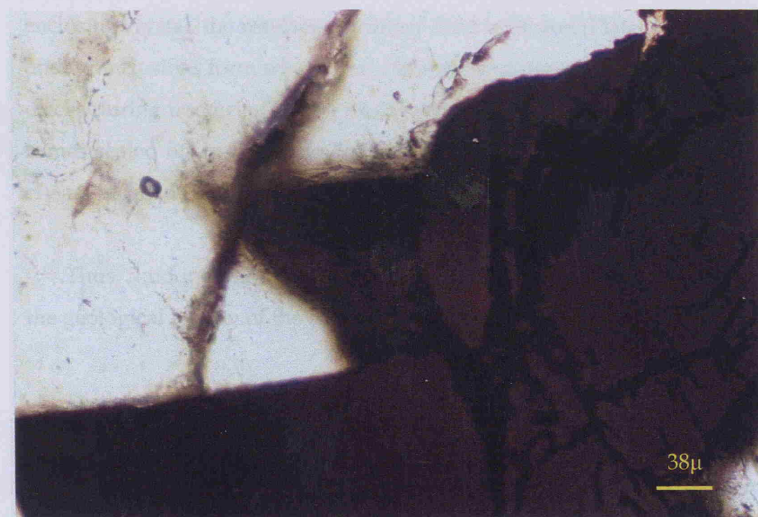
Plate 7.1 : Quartz in textural equilibrium with (a) undeformed (euhedral) and (b) cataclastic arsenopyrite replaced by quartz precipitated in active tectonic environment (shear zone). Random distribution of primary Type I inclusions.
