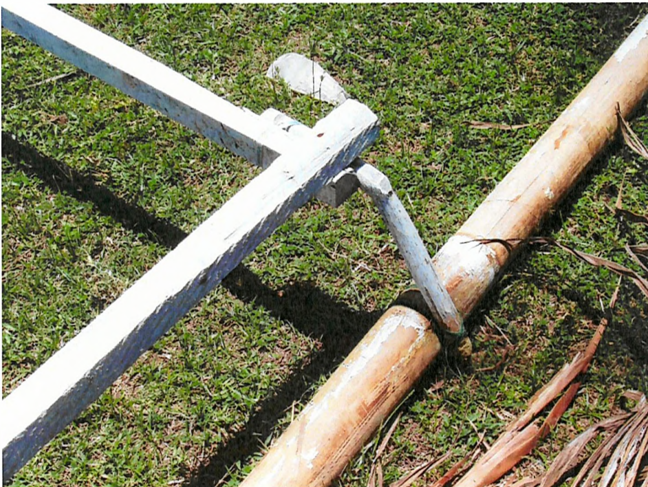
Figure 8.11 The 'elbow' outrigger connection, photo: M R Stead
