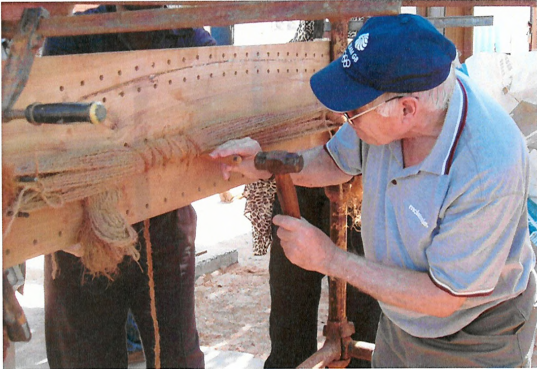
Figure 6.16 An exercise in Arab sewn ship techniques in Oman Maritime, photo: M. R Stead
