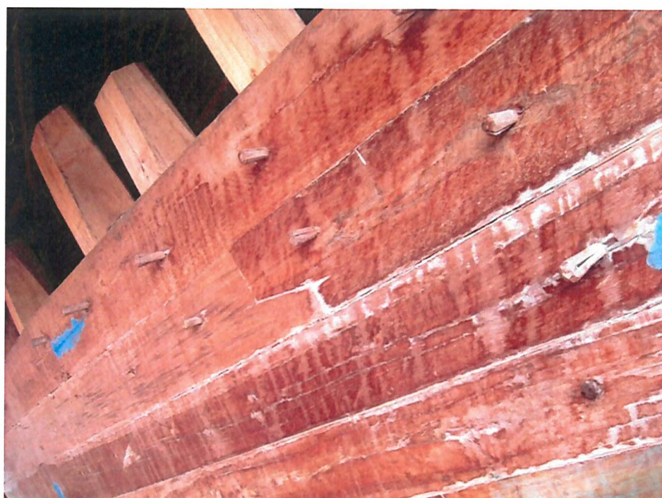
Figure 10.2 The use of treenails in a traditional shipyard in Sulawesi, photo: M. R. Stead
