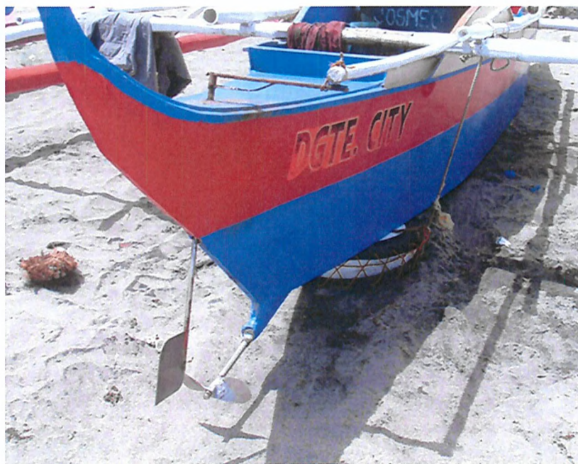
Figure 9.10 Banca in Dumagete with western rudder and inboard engine, photo: M. R. Stead
