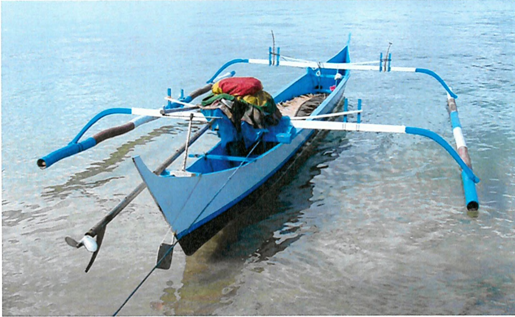
Figure 8.10 The 'bent arm' outrigger connection, photo: M R Stead
