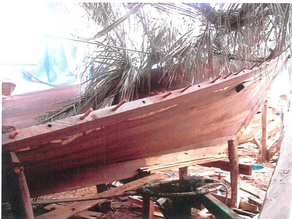
Figure 10.1 The use of dowels for fitting strakes in a traditional shipyard in Sulawesi, photo: M. R. Stead
