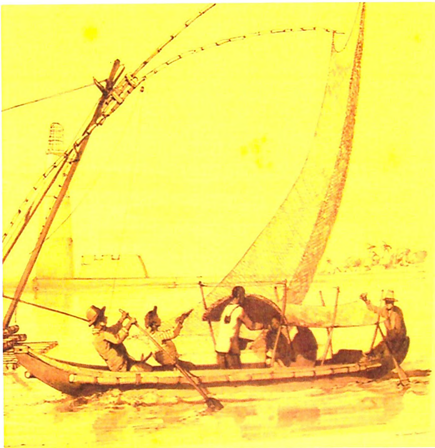
Figure 5.2: Side timbers on a Philippine logboat, from Pâris 1841: Manila banca Pl 75
