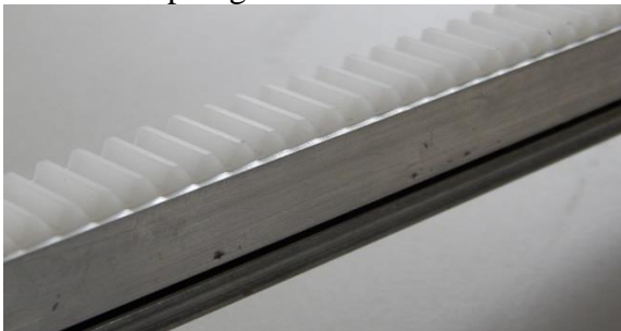
c. Delrin rack housed in the c-channel
