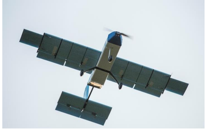
b. Flight testing with wing extended by 30%.
