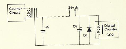
FIGURE A4.14 Block Diagram of the complete counter system.
