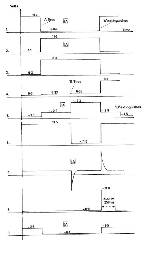
pulse from point 2A to monostable A is removed (Fig. A4.11,9)), thus allowing the positive pulse to fire the monostable (Fig. A.4.11,8)) completing the count as the relay latches during the astable state of monostable A.
