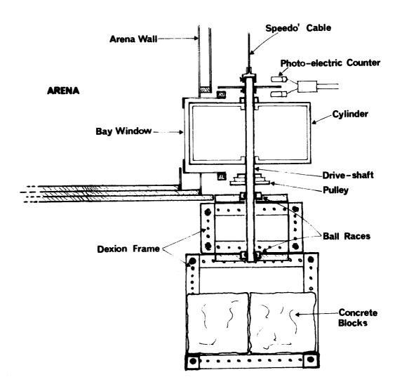
FIGURE A2.5 Block diagram of Arena and Apparatus used in Movement Experiments to show relationships.
