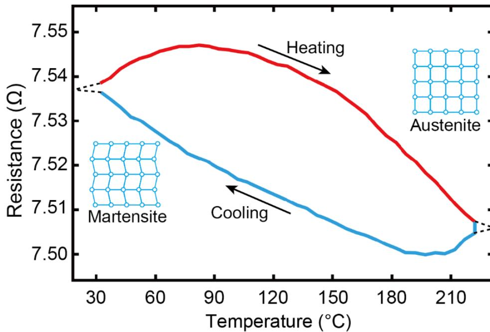
**Fig. 3.** Hysteretic dependence of resistance on temperature for a 175-nm-thick NiTi film on a fused silica ( $\text{SiO}_2$ ) substrate.
