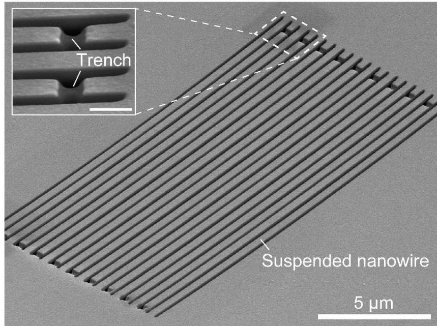
**Fig. 2.** Shape memory photonic nanowire array. Scanning electron microscope image of the nanostructure fabricated on a Au-NiTi-SiN nano-membrane. The inset shows the trenches fabricated at the ends of every other beam (scale bar = 500 nm).
