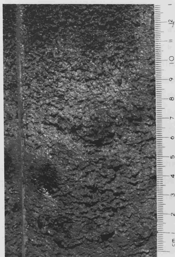
Figure 6.6: Detail from the carbonate cap of a neighbouring core, showing the heterogeneous nature of the surface sedimentary layer.
