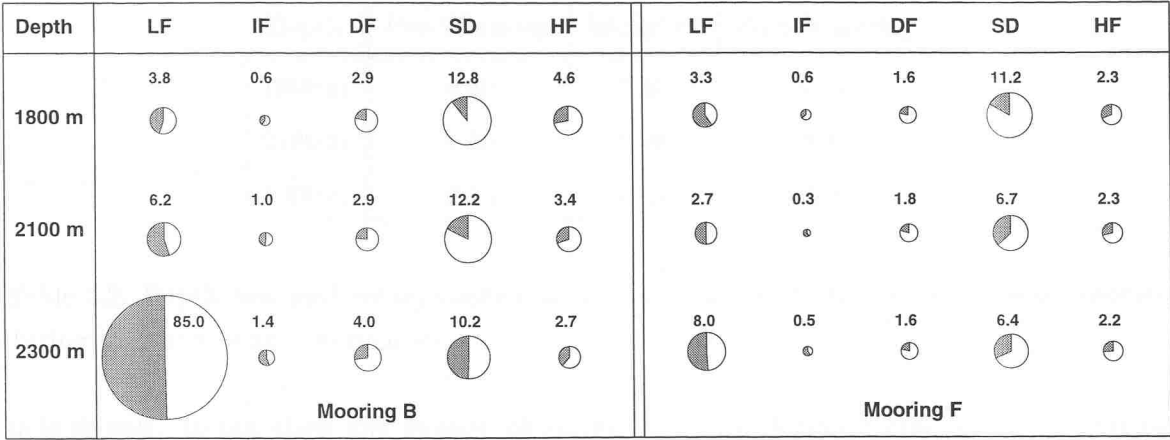
Fig. 4.5: Pre-warming energy partition of the current-meter records of moorings B and F; the limits of the frequency bands are listed in table 4.1; pie areas are proportional to the energies which are also listed in units of 10^{-4} \text{ m}^2 \cdot \text{s}^{-2} above the pies; shading is determined by the relative polarizations with shaded sectors denoting the ACW components.
