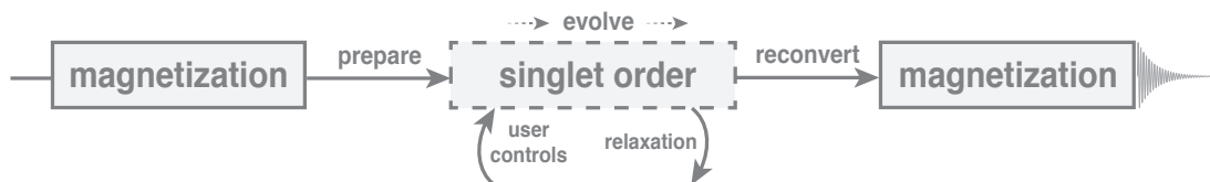
FIGURE 2.13: The three crucial stages of a singlet NMR experiment. Prepare: the spin system is engaged by incoming pulses from the spectrometer which encode the original magnetization as a more preferential form of spin order where relevant information is consequently stored. Evolve: the newly established spin order is propagated forward in time under the influence of coherent effects (including user defined control such as continuous wave rf-fields and pulsed field gradients) and incoherent relaxation phenomena. Reconvert: NMR experiment detect physical observables, such as the \hat{I}^- operator, and as such reconversion to observable magnetization is required for monitoring the evolution and relaxation of the established spin order.
