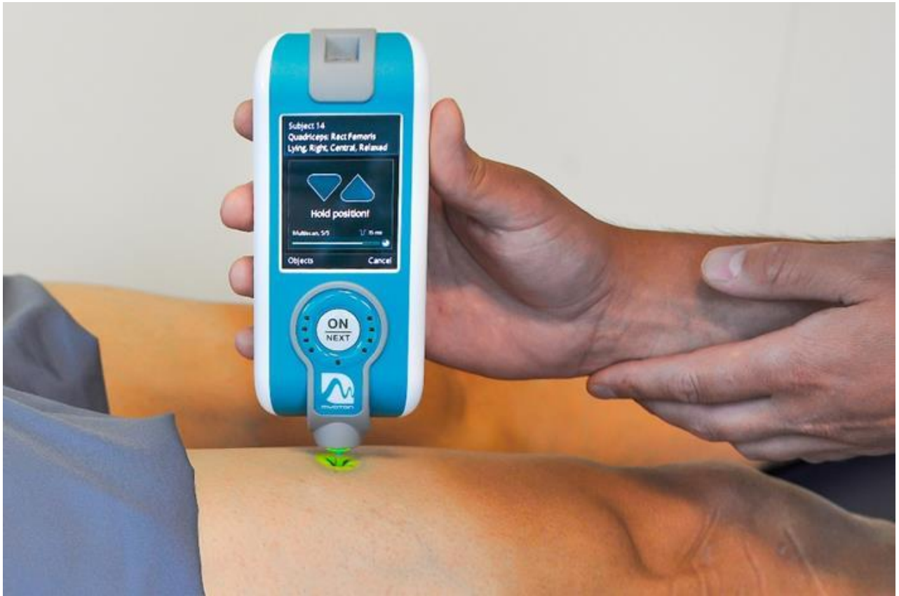
Figure 2. MyotonPRO technique for measurement of rectus femoris (RF) stiffness, tone and elasticity. The device probe is held perpendicular to the skin for accurate recordings
