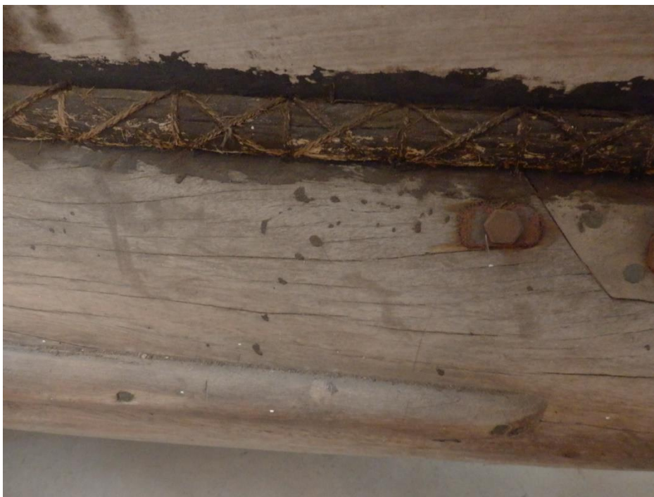
Figure 90 Stitches used on a full-size oru . In the National Maritime Museum Cornwall collections (National Small Boat Registration number 383, photograph taken by Charlotte Dixon, 2017)
