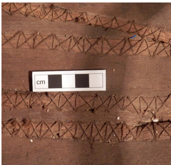
Figure 24 Close up of masula boat model from Figure 23 showing the stitching. It shows the inboard of the model with the stitches forming a criss-cross pattern used to join the wooden planks together. In the EISCA collections (No inventory number; photograph taken by Charlotte Dixon, June 2014)
