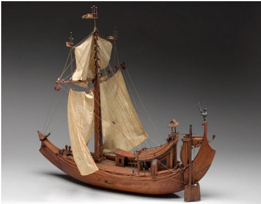
Figure 172 Model of an Irrawaddy rice boat with a bipod mast. In the Science Museum's collections (inventory number 1894-184; © Science Museum / Science & Society Picture Library -- All rights reserved. http://www.scienceandsociety.co.uk/ accessed on 11 th June 2014)
