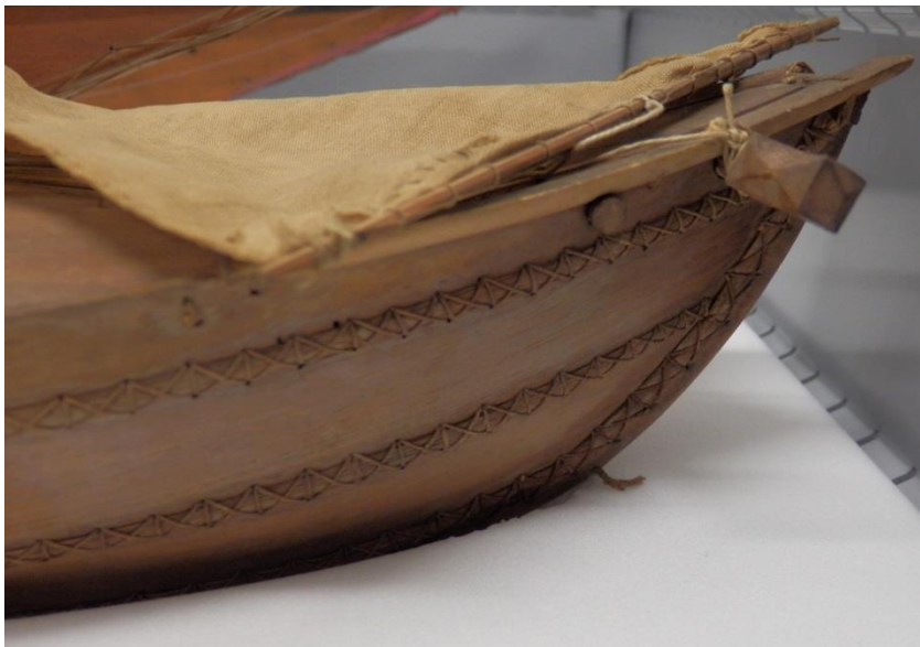
Figure 86 Sewn technique applied to a model of a yathra dhoni . In the British Museum collections (inventory number As1933,1110.1; photograph taken by Charlotte Dixon, 2014)
