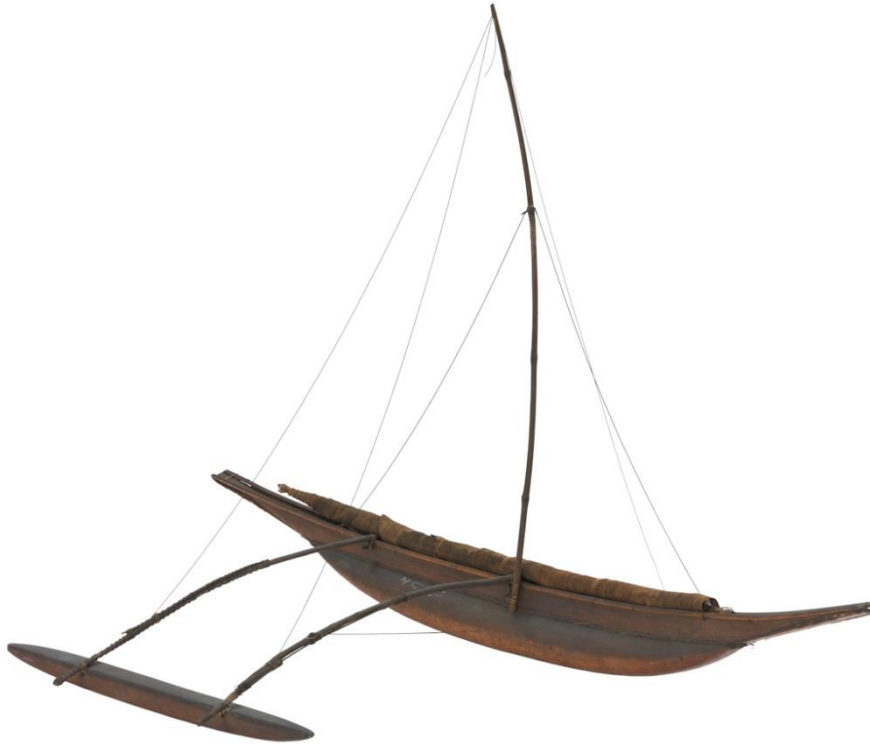
Figure 51 Model of an extended logboat with a single outrigger. The planks have been sewn to the hull and there is a mast and furling sail. In the National Maritime Museum collections, 13680mm in length (inventory number AAE0006; © National Maritime Museum, Greenwich, London)
