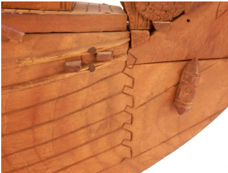
Figure 156 Model of a Burmese boat with incised planking and scarf join at the stem. In the Pitt Rivers Museum collections (inventory number 1969.8.6; photograph by Charlotte Dixon, 2015)
