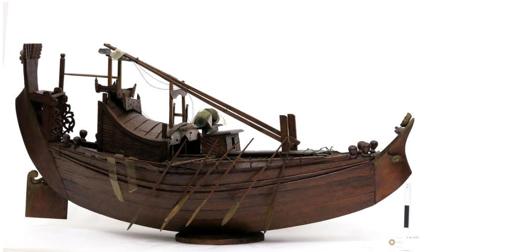
Figure 155 Model of a laung-zat for transporting rice. It is made from flush-laid, planking with additional stem and stern posts. This model also has an oculus (eye) at the stem. In the Horniman Museum and Gardens, 1016mm in length (Inventory number 1975; Horniman Museum and Gardens)
