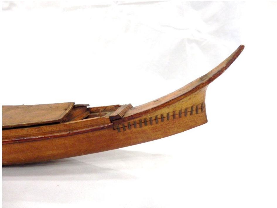
Figure 154 Model of a sat lay for rice transportation. It was commissioned for the Glasgow International Exhibition, 1888. There are metal staples at stem and stern joining the hull with stem and stern posts. In Glasgow Museum collections (inventory number 1888.109.ul; photograph by Charlotte Dixon, 2015)
