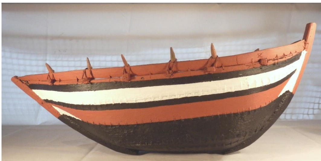
Figure 23 Model of an Indian masula surf boat. It has been made from a series of wooden planks sewn together and depicts different patterns in the stitching inboard and outboard. In the EISCA collections, 630mm in length (no inventory number; photograph taken by Charlotte Dixon, June 2014)
