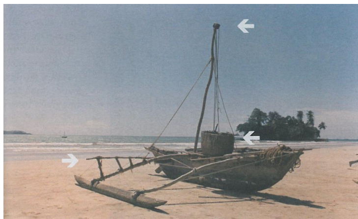
Figure 60 A large palu-oru for tunny fishing offshore. Note the masthead block, the horizontal timber on the after outrigger boom and the fish basket (all arrowed), Weligama Bay, 1986 (Kapitän et al., 2009: Fig. 137)
