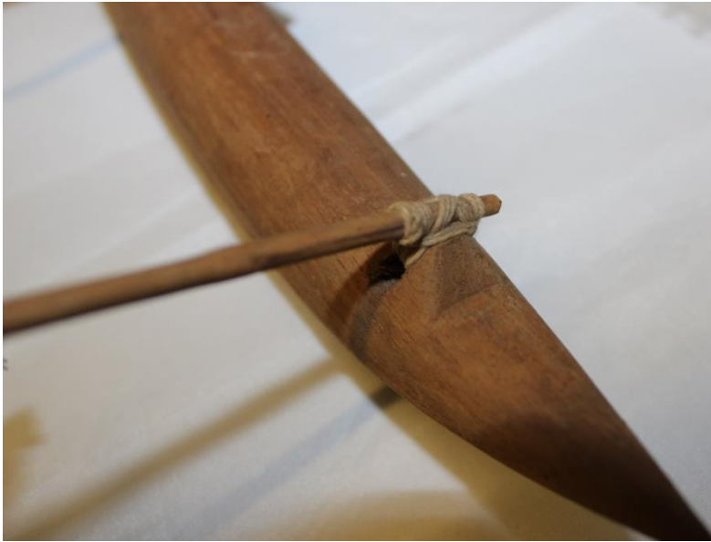
Figure 92 Model oru with a raised section in the outrigger float for attachment to the outrigger boom (inventory number AAE0158; with kind permission from the National Maritime Museum, Greenwich, London)
