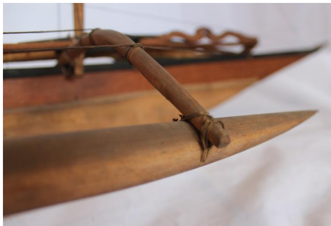
Figure 91 Holes are bored into the outrigger float and lashed to the boom, as demonstrated in this image of a model from Southampton City Council Arts and Heritage collections (inventory number temporary number 2; photograph taken by Charlotte Dixon, 2015)
