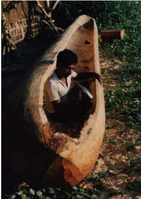
Figure 64 Hollowing out a log with an adze (Kapitän et al., 2009: photo 39)
