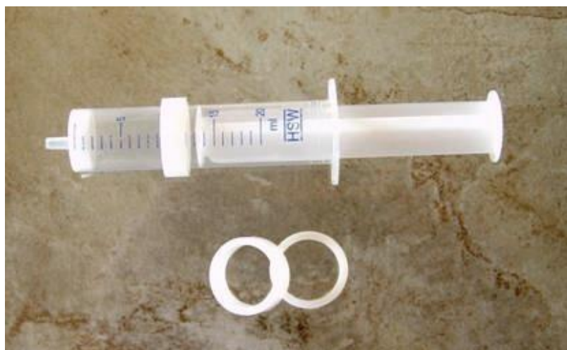
Figure 3-16: Reactor used for manual solid phase of PNA. 180
