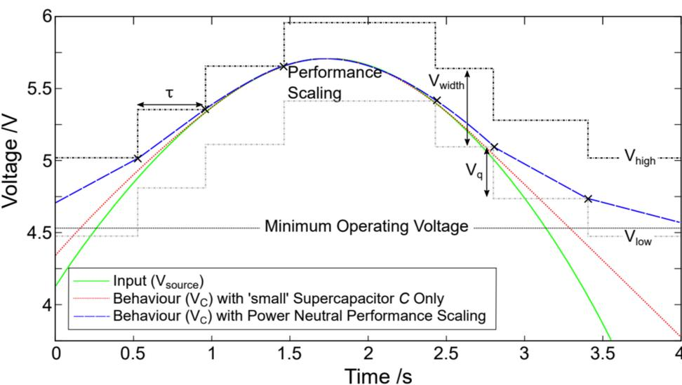
Behaviour of an EH system to a transient input (green), with (blue) and without (red) power neutral performance scaling
