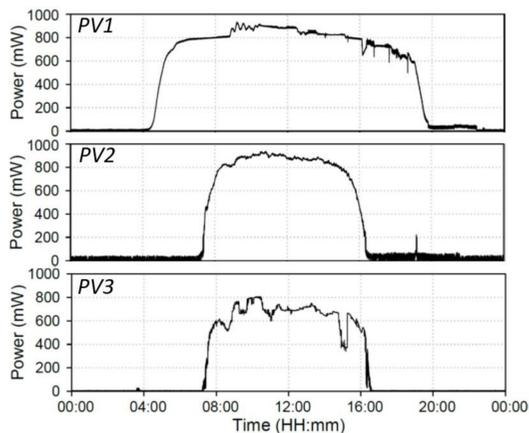
Power outputs from three PV cells located outdoor
