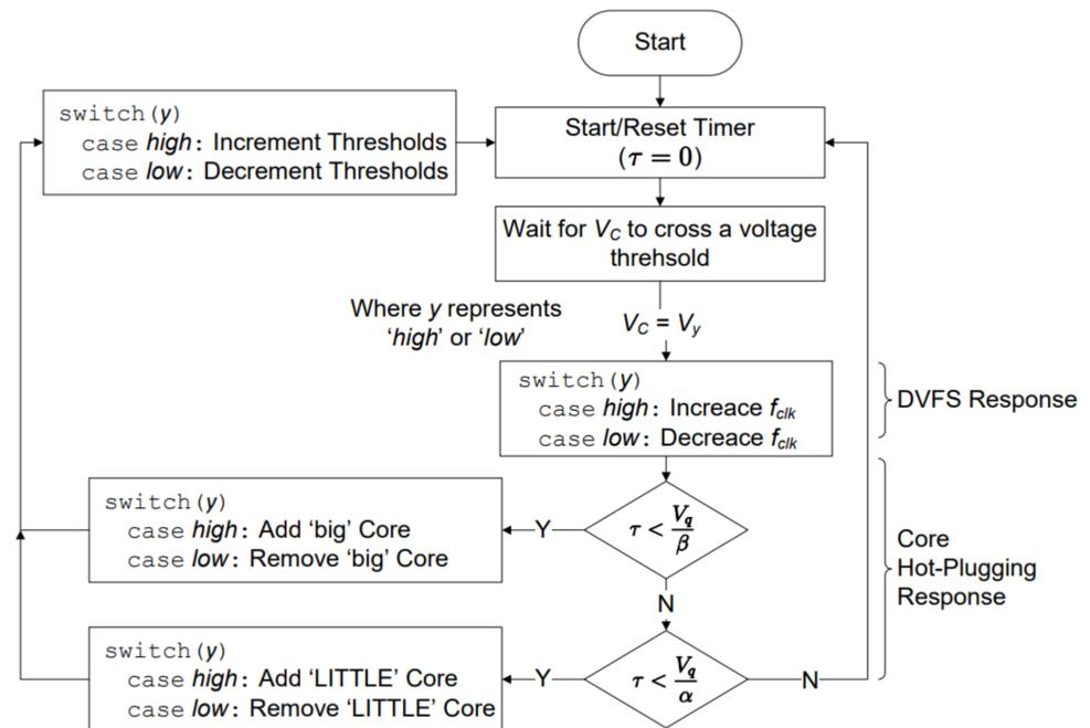
Flowchart depicting the principles of the power neutral performance scaling approach using DVFS and core hot-plugging
