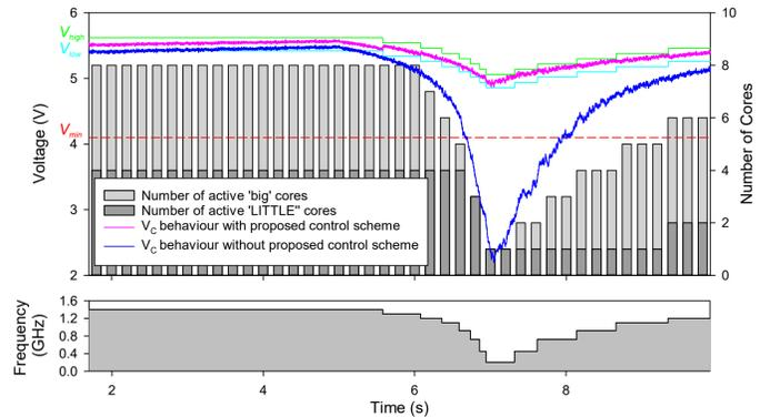
Fig. 1. Simulation of operation under power neutral control scheme [2].
