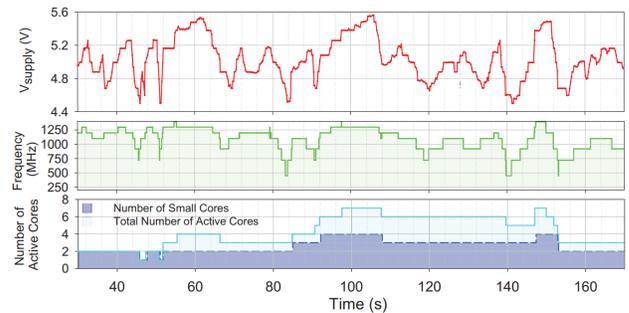
Fig. 2. System performance using a controlled voltage supply [2].
