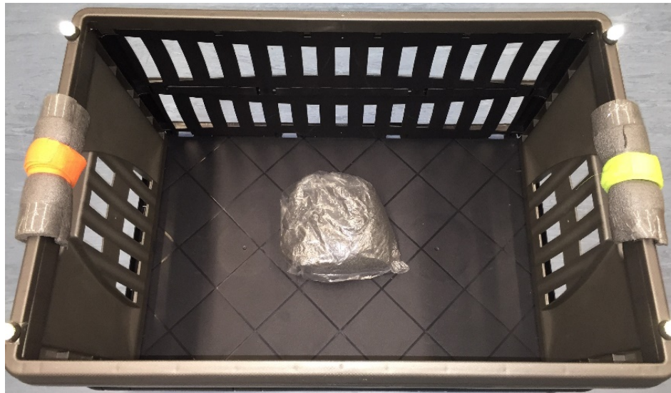
Figure 3.6. Foam-fitted plastic container with 1kg load (sand bag)
