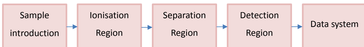
Figure 1.34 - Schematic depiction of a generic ion mobility spectrometer
