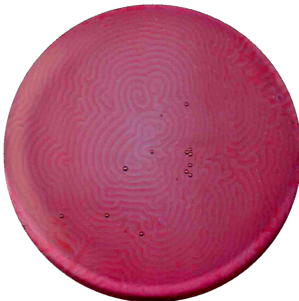
FIGURE 3.1: Pattern formation in the unstirred BZ reaction. Spiral waves and planar wavefronts are visible along with bubble formation in a reaction set up in a petri dish. Image colour has been enhanced for clarity.
