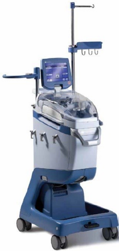
Figure 3. Autologous Cell Saver. Cell savers perform a similar role to the cardiotomy suction; blood from the surgical field is sucked into the reservoir where it is sent to a "Latham bowl". The spinning of the bowl creates centrifugal force pushing the heavier red blood cells to the bottom and the lighter plasma to the top. Once full of red blood cells, saline is pumped into the bowl to wash lysed red cells into a waste bag. When the blood is "clean" (as assessed by the level of plasma free haemoglobin) the red blood cells are sent to an autologous blood bag where it can then be re-infused directly into the ECC or the patient. Image supplied by LivaNova and reproduced with Permission.
