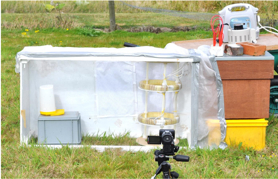
Figure 64. Flight cage attached to the front of a nucleus hive. A feeder is located at the far end of the cage. The Helmholtz coil and stand are placed between the hive and feeder such that bees must fly past the Helmholtz coil to reach the feeder, and to return from the feeder to the hive.
