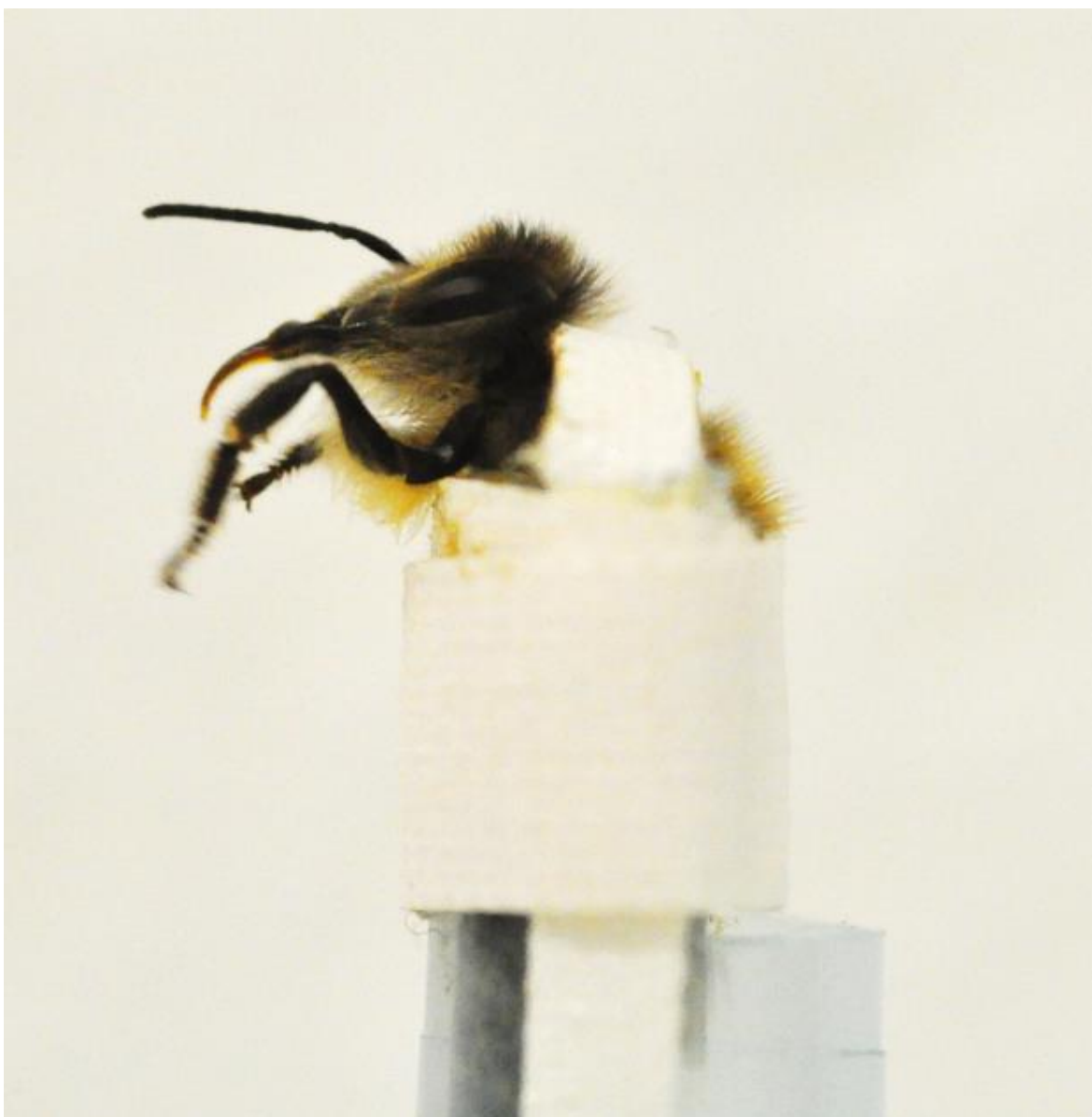
Figure 37. Harnessing of bee in PER tube for stress protein experiments and appetitive associative learning experiments. Tesa tape was wrapped over the thorax around the back of the head, to hold the bee in place, whilst allowing the bee free movement of the head, antennae and forelegs.
