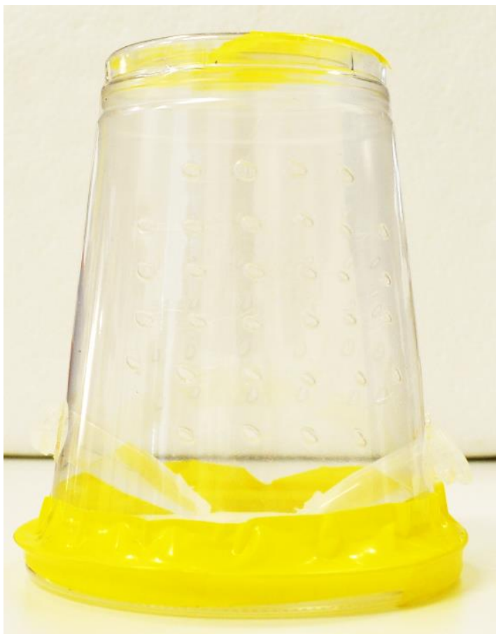
Figure 59. Disposable cage used for collecting bees and keeping overnight in tethered flight analyses. Two 1.5ml Eppendorf tubes were placed within the cage with holes for feeding, containing 40% w/v sucrose.
