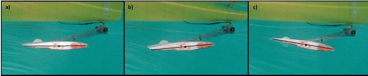
Figure 19: Forward foil spring loaded motion: a) Neutral Angle b) Positive Pitch c) Negative Pitch
