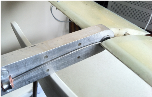
Figure 7: Pivot arm and rotational spring setup
