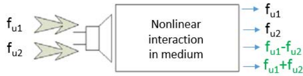
Figure 2-17: Non-linear interaction process in air (frequencies in green font produced by non-linearity) after Wen-Kung,T [39]
