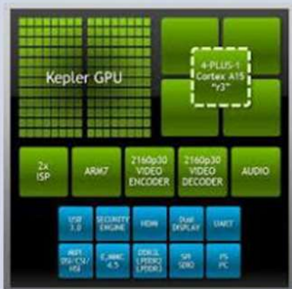
Nvidia Jetson TK1 - Quad core CPU + 192 cores GPU
