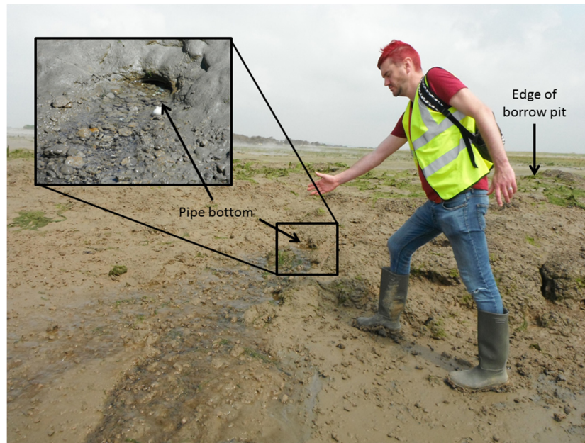
Fig. 7. Water flowing from the bottom of a pipe (inset) through the bank of the borrow pit in June 2014.
