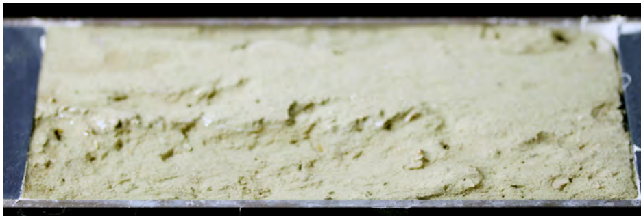
(c) Eroded sample at a density of 1707 \text{ kg/m}^3 with a constant shear stress at \sim 2.3 times the threshold showing mainly artefacts of mass erosion.
