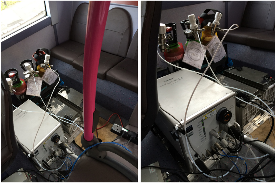
Fig. 6. PEMS equipment installation on the test bus.
