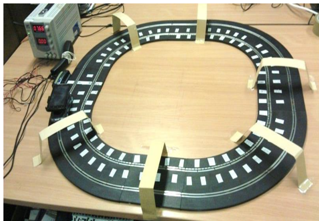
Figure 3.4: A slot car ‘Scalextric’ racing track powered by a DC voltage supply with smartphone mounted on top of the toy car kept at the top left. The track consist of several curved and straight edges with temporary bridges placed at some distance apart from each other.
