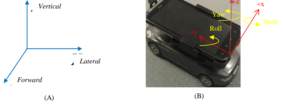
Figure 3.2: (A) Global Coordinate System (B) Smartphone's Coordinate system
