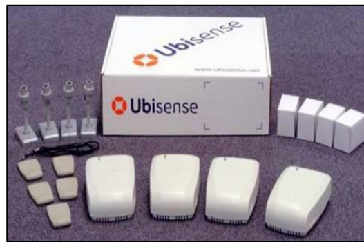
Figure 2.12: Hardware of the Ubisense System in an Academic Research Package: five tags (left) and four sensors (right) (Source: [53]).
