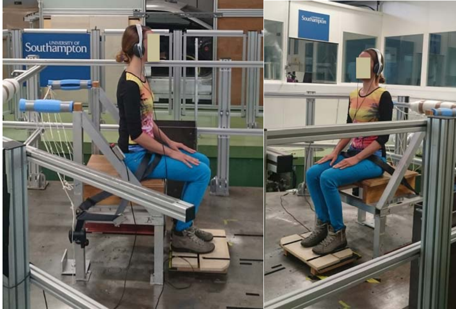
Figure 2 Experimental setup on the 6-axis simulator.
