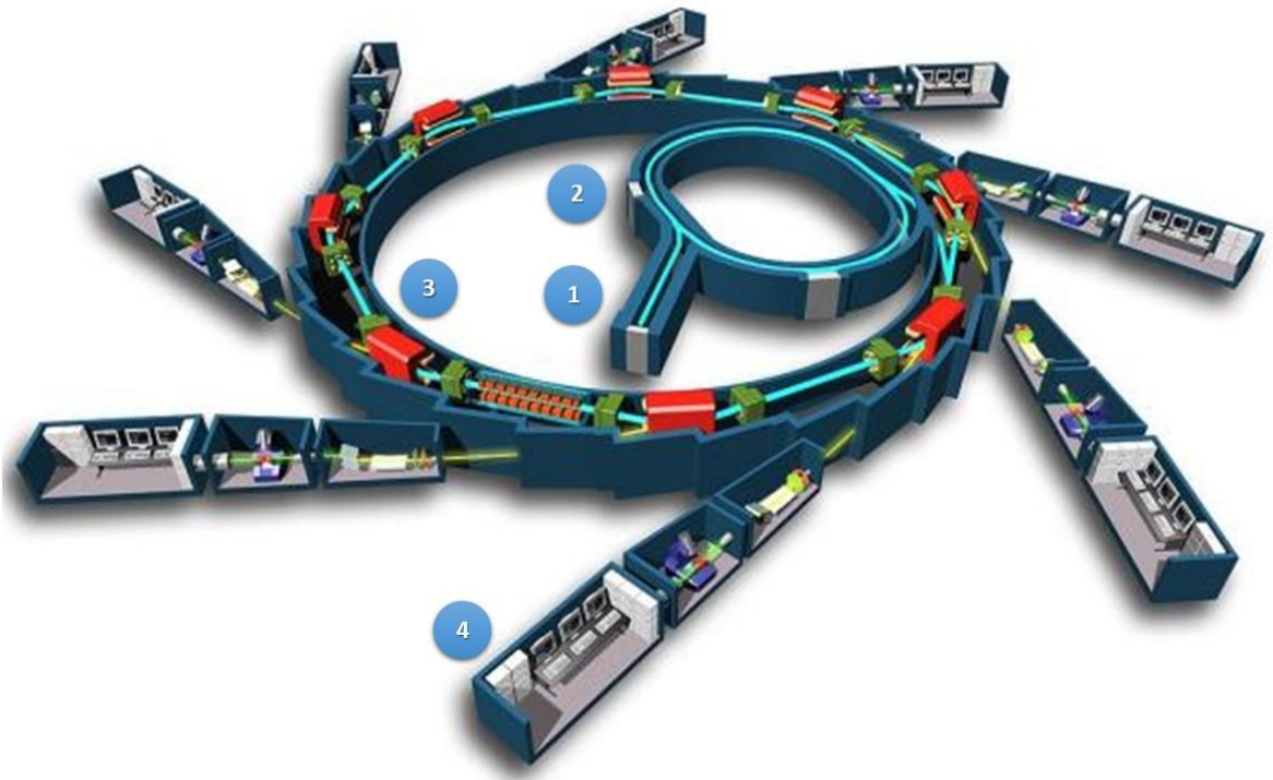
Figure 2.3. Synchrotron technology. Electrons are generated (1), accelerated (2), deflected through electromagnetic field in the storage ring (3) to create extremely bright light. Light is channelled down beamlines to workstations (4) where it is used to scan the samples.
