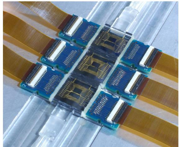
**Fig. 1.** Three modules of our modular, reconfigurable quantum circuits are connected to build a large and programmable multiport interferometer with 20 inputs and outputs. This three module device is glued to two fibre V-groove assemblies and the phase shifters are controlled via electrical ribbon cables. The connectivity of the interferometer is determined by the number of modules.
