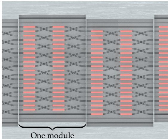
**Fig. 2.** A rendered impression of concatenated modular chips. The phase shifters are shown in red, and the waveguide pitch has been exaggerated for clarity. Each second chip is offset by one waveguide (127  $\mu\text{m}$ ) to form a multiport interferometer.
