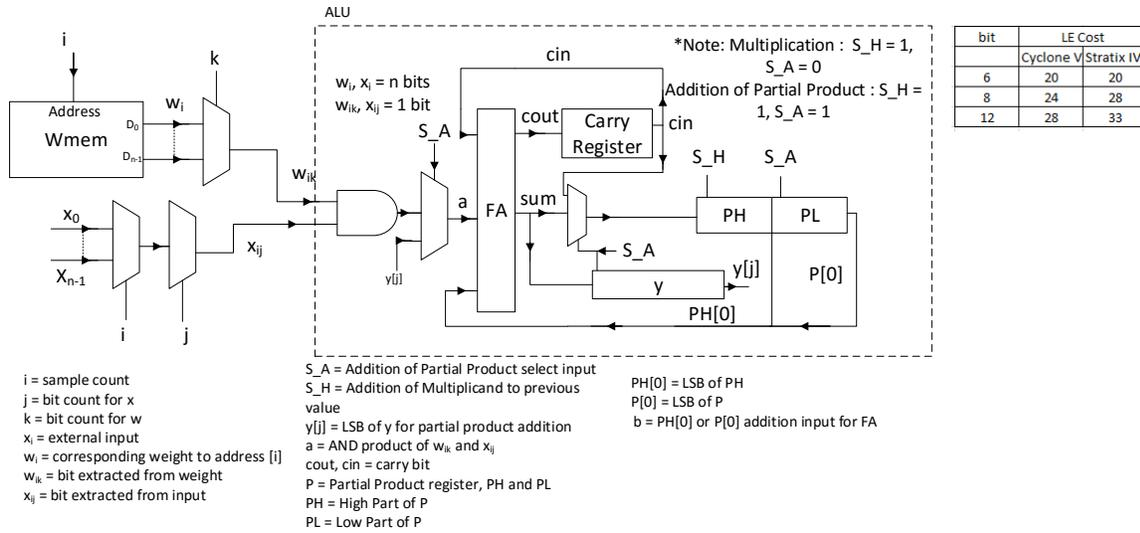
Fig. 1: DPU Design (Logic element counts are included in table) [3].
