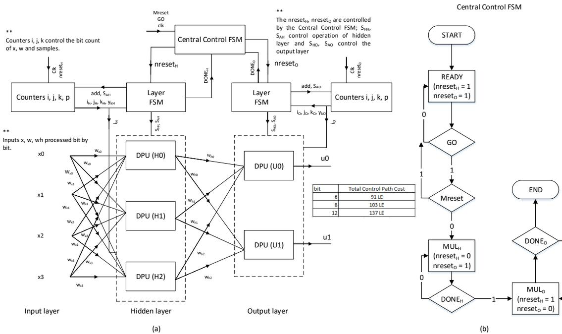
Fig. 2: (a) Hardware topology of the proposed implementation of a multi-layer perceptron, (b) Central control FSM chart.[3]
