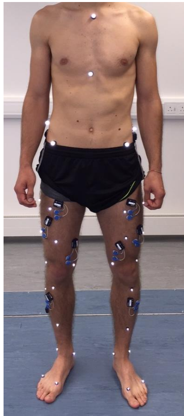
Figure 1: Anterior view of reflective marker placement for motion capture and EMG placement.
