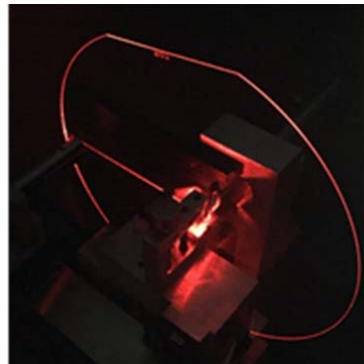
Figure 89. Image of the light guiding quality of the SiON film on a borosilicate substrate at 633nm. The image shows the Metricon prism coupling system with a red streak of guided light.
