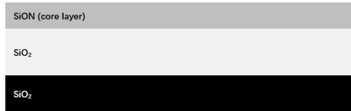
Figure 21. Cross section of the SiON/SiO 2 /Si slab waveguide structure.
