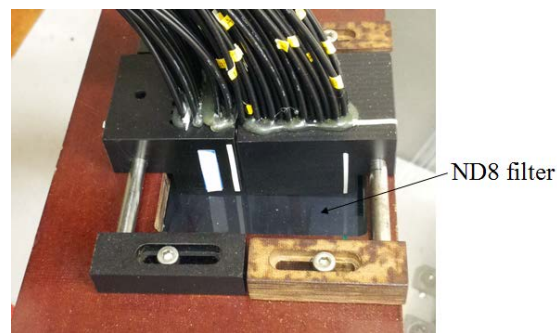
Figure 156 Filter between a fibre array block and outer glass.
