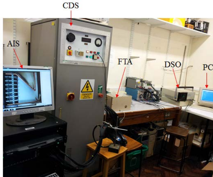
Figure 58 Overall set-up of the arc imaging test.
