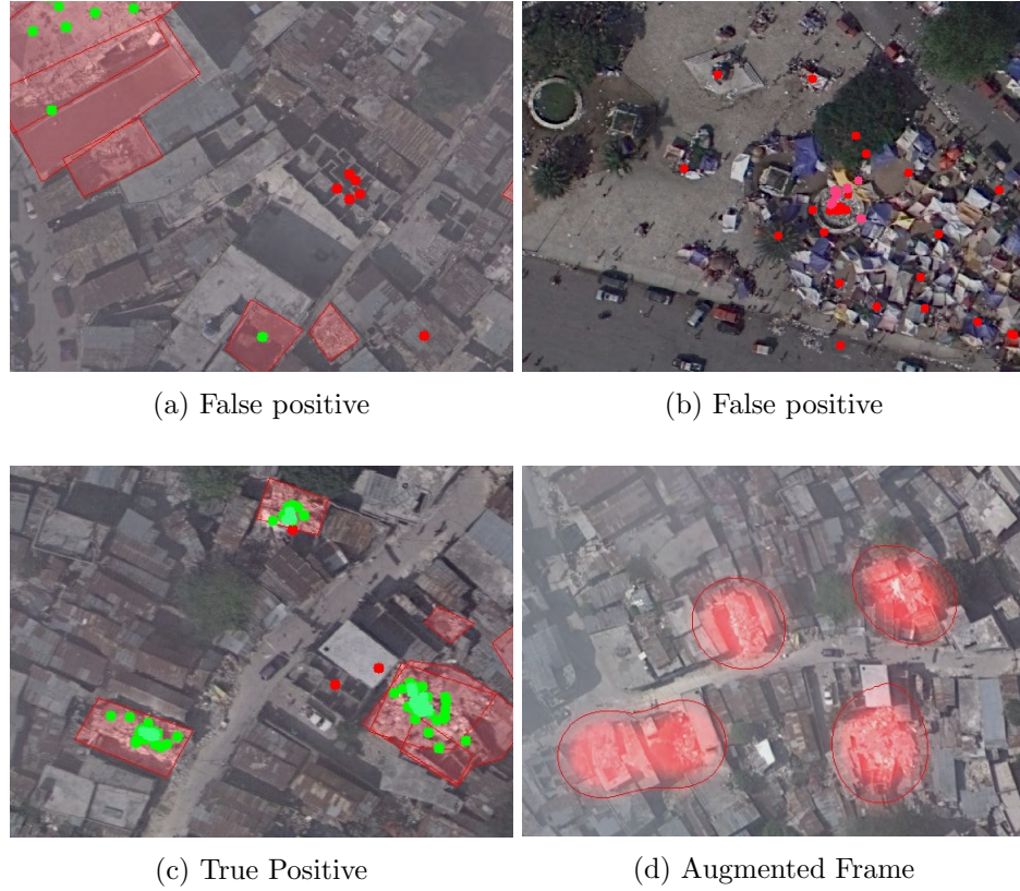
Figure 5.14: Examples of true and false positives, worker clicks are colored in green (correct) or red (incorrect). In (d) we can see an example of the augmented output, with identified clusters colored randomly.
