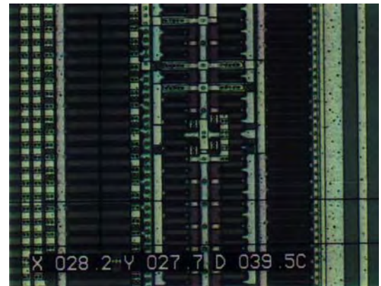
Figure 4.4: Op-amp metallisation on untreated die. (Original in colour)
