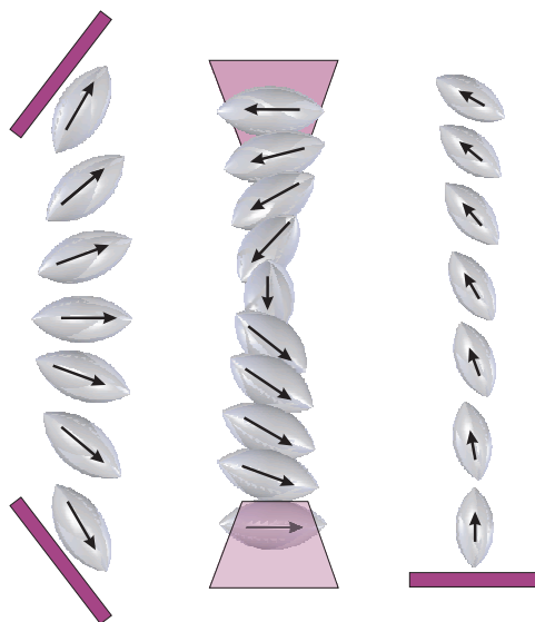
Figure 10.3: Representation of the splay, twist and bend deformations (left to right respectively). Each 'bead' represents the director orientation.
