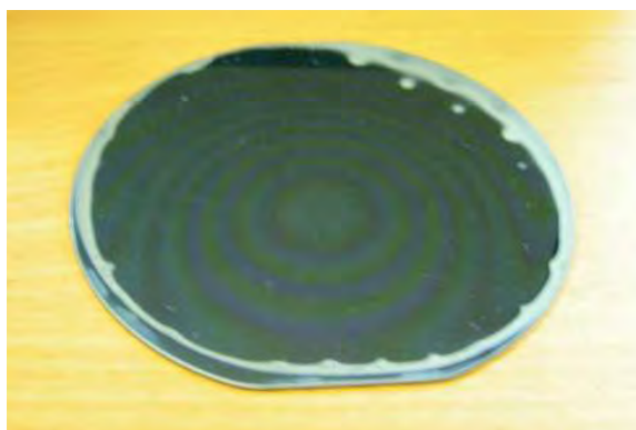
Figure 6.18: A sample demonstrating layer pullback from the wafer edge. In this case layer 11 (see table 6.2) was deposited on layer 8. Slight bubbling was also present over the whole wafer.
