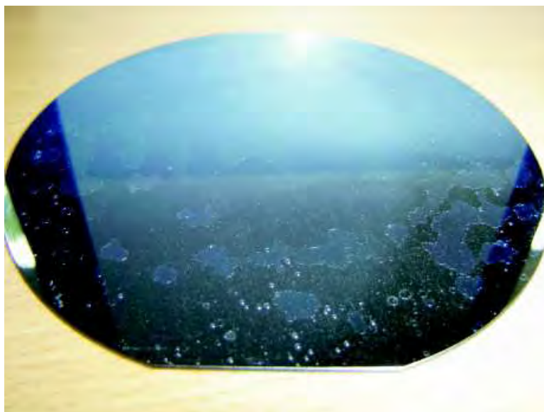
Figure 6.5: Wafer showing delamination and bubbling after annealing
