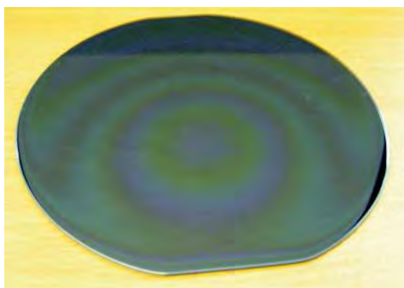
Figure 6.21: A 6 micron layer of the final recipe, germanium doped core layer.
