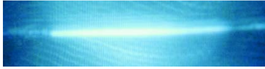
Figure 12.10: Intensity profile of the TM_0 mode at 1.536 \mu\text{m} at the output of the waveguide.
