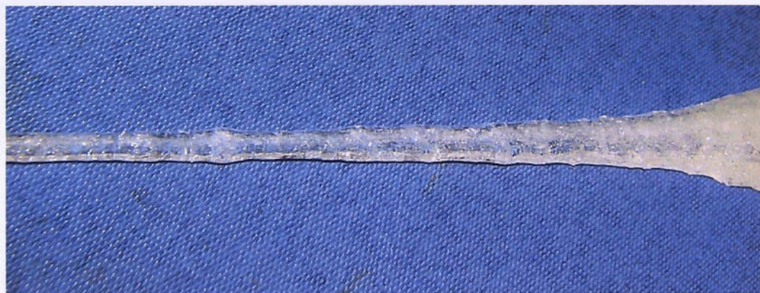
Figure 6.19: The result of a trial attempt at pulling a fibre from the YAS3 sample. The glass is heavily devitrified.
