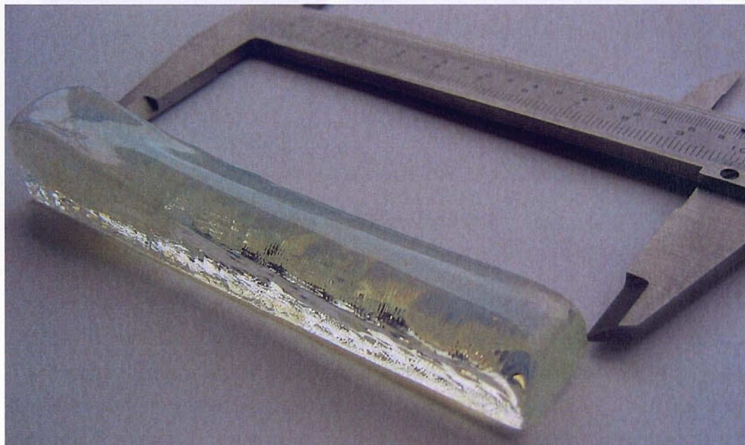
Figure 6.16: 10 cm long YAS glass bar used for the preform for the unclad fibre.
