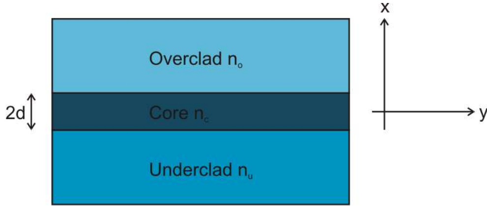
Figure 3.6: Structure of the asymmetric slab waveguide. The structure is continuous in the y and z axis with the refractive index varying in the x direction. The refractive indices of the structure are n_o , n_c and n_u where n_c > n_o, n_u and the thickness of the core is 2d .
