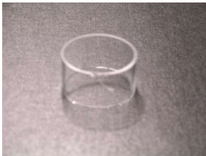
Figure 5.11: Fully consolidated planar layer on the outside of a cylindrical substrate deposited through the FHD process.
