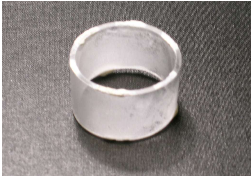
Figure 5.9: Cylindrical silica substrate crystallised after 1400°C consolidation process.
