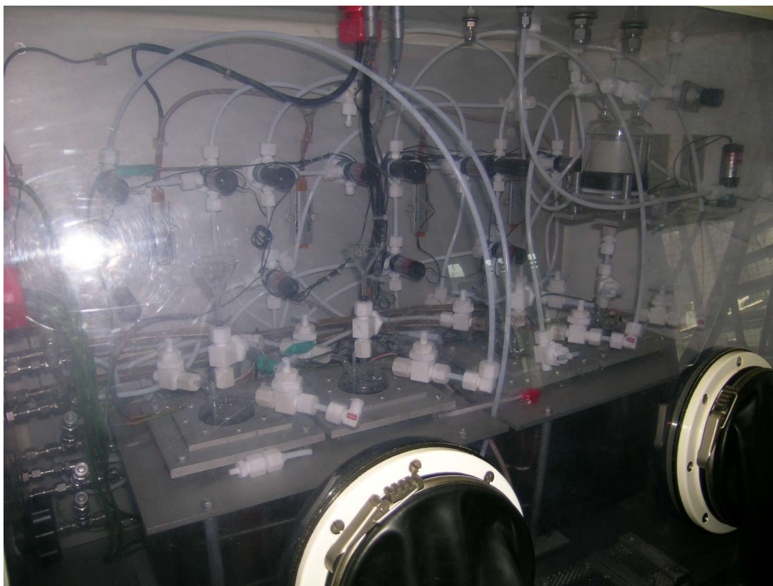
Figure 5.4: Picture of the reagent delivery system for the FHD system.
