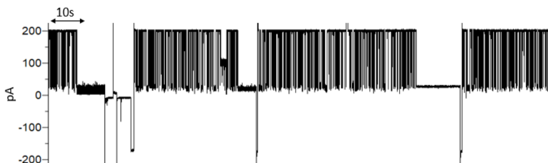
Figure 6.3. The representative current trace of \alpha\text{HL} pore for 0.5 / 4 M KCl gradient in the presence of 20 nM miDNA155, 100 nM P155 and 0.27 \mu\text{g/mL} of total RNA extract from blood serum sample
