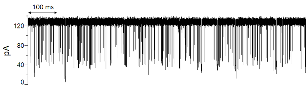
Figure 3.14. Single channel current trace in the presence of 0.5 mg/mL PEG 1000 in 4 M KCl solution at +30 mV.
