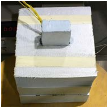
Fig. 3. Concrete cube in the polystyrene box.
