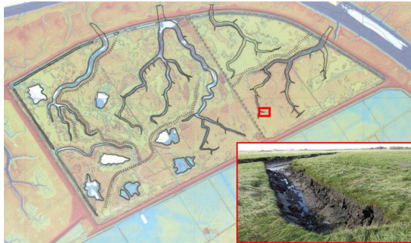
Figure 8.3: Channel “grip” at Hesketh Out Marsh East, August 2017. Lidar image courtesy of Richard Shirres.
