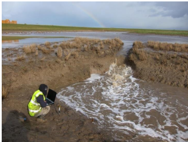
Figure 8.5: Ebb flow routing through pre-excavated channel head tributary at Steart (Photo taken by Anas Annar, 23/02/2015). This has continued to expand, leading to secondary channel formation into the adjacent marsh.
