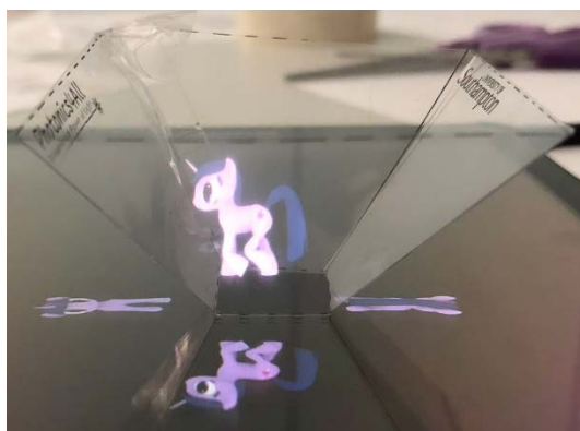
Figure 1: Demonstration of the “Mobile Ghosts” activity using a tablet. The pyramidal 3D projector is made from a net printed on a sheet of acetate, so they are cheap to reproduce and students can take them away after the workshop.
