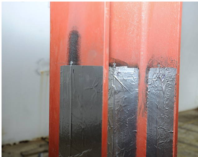
Fig. 6. Endevco 8515C-50 surface pressure transducers mounted on Specimen A.
