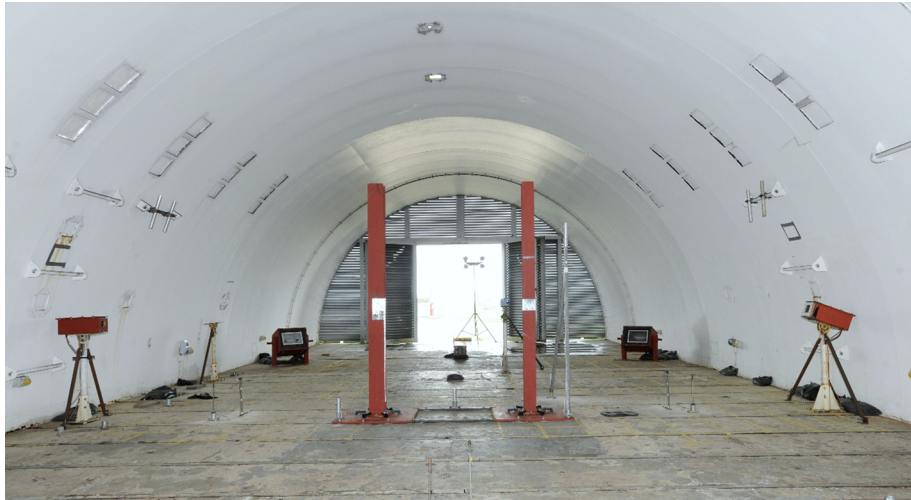
Fig. 3. Trial configuration in the ABT viewed downstream for the 0° I-section orientation (Trial 1).
