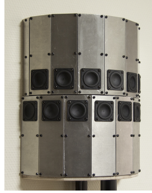
Figure 13: (Colour online) Prototype of a HCA with r_S = 14.2 cm and L = 15 Tang Band W1-1070SG full-range drivers.
