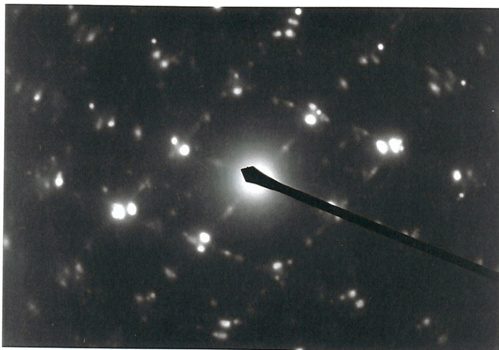
Figure 4.18: Material 'C'. Heterointerface. (110) electron diffraction pattern.
