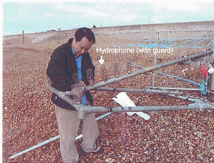
Figure 5.12: Photograph of the hydrophone array used in the second sea trial. One of the experimenters (Mr. Yim) makes final adjustments to the rig prior to deployment. Note the wire gauze around each hydrophone to protect it from impact with wave-borne stones. Also to the right of the image the edge of the acoustic source and water-tight canister can be seen. In the background the 200m (blue) umbilical cable has been paid out ready for deployment.
