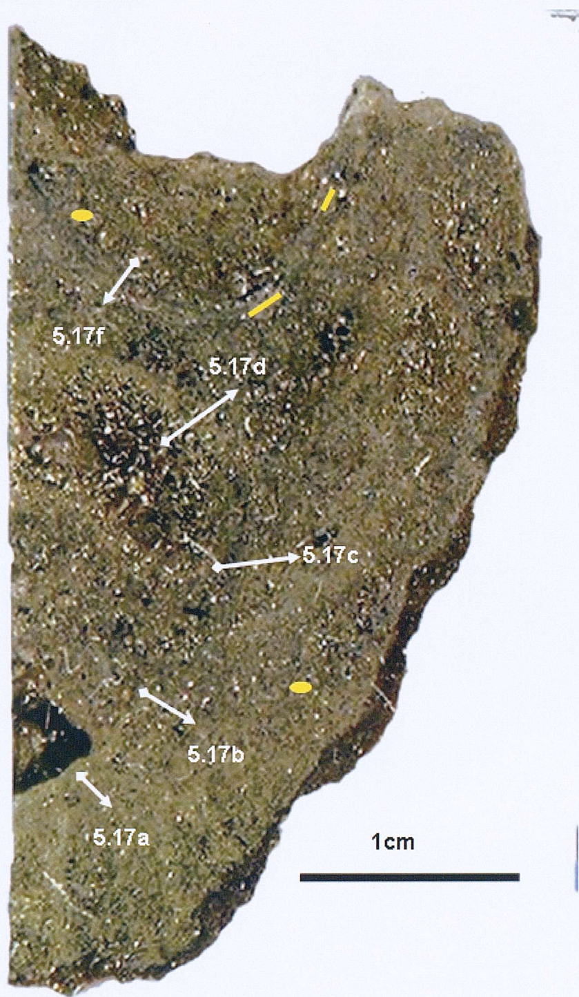
Figure 5.8 – EPR 99 01 A (partially infilled tube from figure 5.6'b' is orientated at top; infilled tube 5.6'c' is located towards mid-left) EMP scan-line traverses marked with white arrows; isotope analysis marked with yellow dots (cpy) and lines (py).
