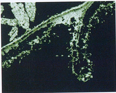
Figure 6.21 - Elemental map for silica.
