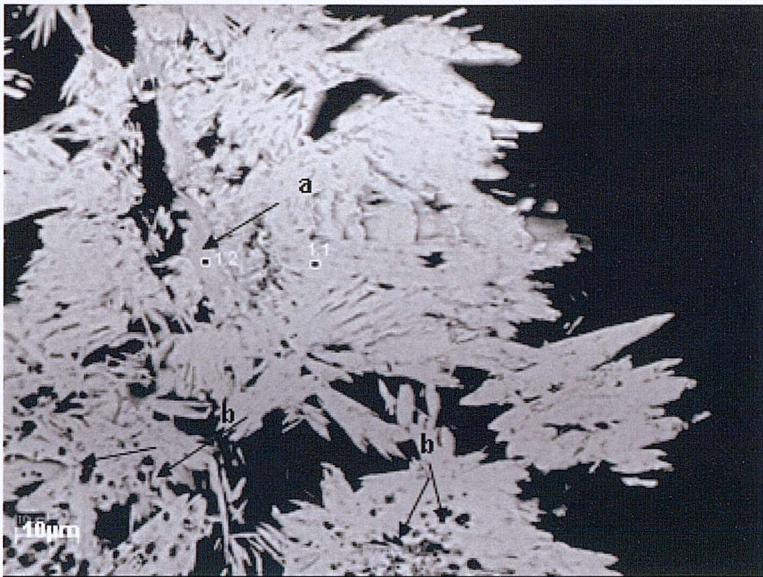
Figure 6.19a (left) – Image located around the end of a terminal flange shows extensive barite mineralisation. ‘Arrow a’ shows the tip of the flange structure, which has been replaced by barite. Arrows b indicate inferred microbial cell ghosts within the barite precipitates encrusting the flange tip. Point analyses shown in later figures.
