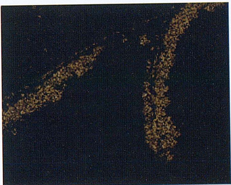
Figure 6.21 - Elemental map for phosphorous.
