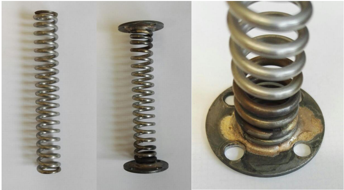
Figure 81: Spring as it appears before (left) and after (central) the modifications and zoom of the welded coil (right) - the holes through the disc allow the fastening with screws
