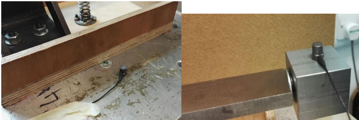
Figure 76: Accelerometer 1 attached onto the base (left) and accelerometer 2 attached onto the lumped mass (right)
