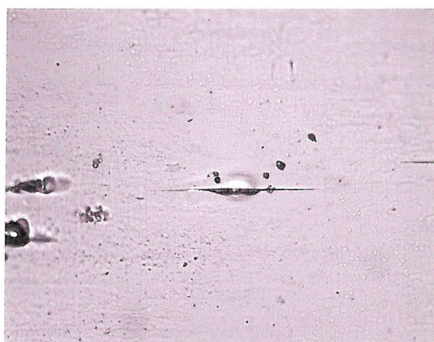
Figure 5.40: Sequence of optical micrographs from acetate replicas showing initiation of Crack III from test A600-750-1-PR-01. The development of bulge-like feature at the initiation site can be seen.
